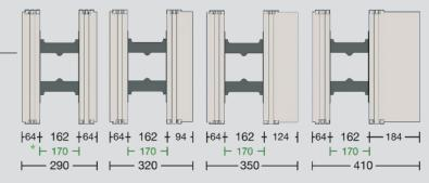
Climablock cross section with 19.2cm of concrete space
