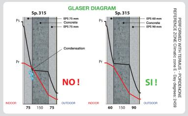
Internal conditions: Temperature 20 ° - Relative humidity 52% - Adductance 7.7 External conditions: Temperature -5 ° - Relative humidity 57.5% - Adductance 25
